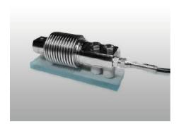
±1% del carico nom. SENSIBILITÀ NOMINALE: ±0.02% a carico nom SBILANCIAMENTO DELLO ZERO: CREEP (20MIN): ±0.02% del carico nom NON LINEARITÀ, ISTERESI E 350ohm  $\pm 4$ ohm NON RIPETIBILITÀ: 350ohm  $\pm 4$ ohm IMPEDENZA DI INGRESSO: -10°C a 40°C RESISTENZA D'USCITA: CAMPO DI TEMPERATURA COMPENSATA:  $^{\pm 0.02\%}$  F.S./ $^{10^{\circ}}$ C DERIVA DI ZERO IN TEMPERATURA:
